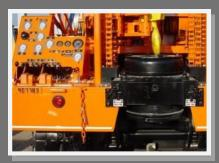
**8-1/2" ROTARY TABLE:** Consists of spiral bevel gear type rotary table enclosed in oil bath case with 8 1/2" diameter opening (6 1/2" sq. opening with master drive bushing), hydrostatic drive, 4-speed transmission, table mounted in a sliding frame which can be hydraulically retracted 18"; 4 1/4" diameter fluted Kelly with drive keys and bushing, and Kelly mud bucket.
